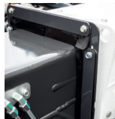
Dust protection on boom
